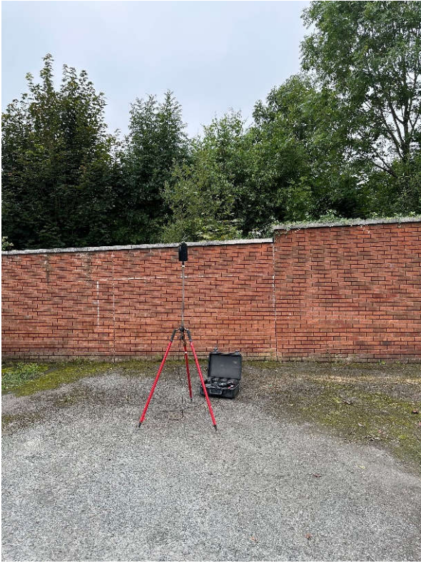
Plate 8-1 Baseline Noise Measurements setup at N1
