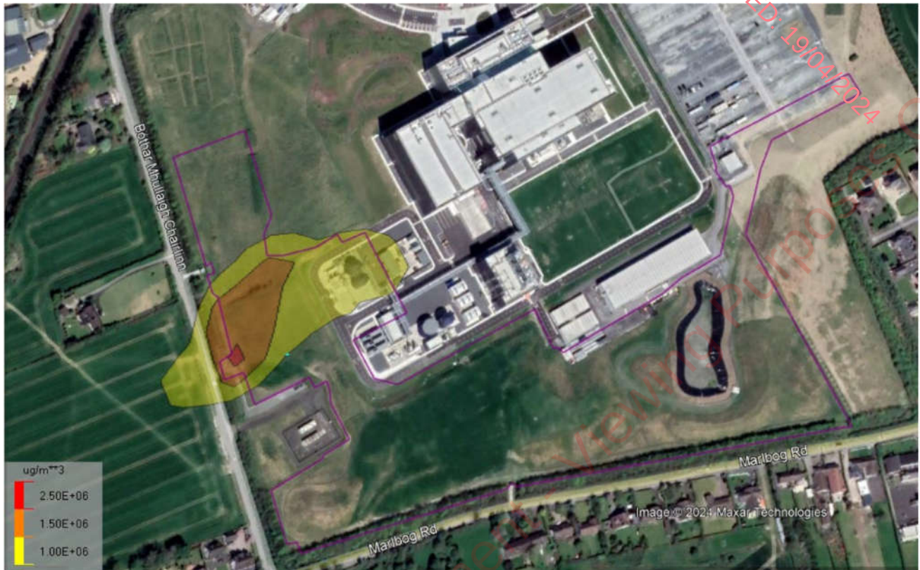
Figure 7.5 67- Isopleth showing maximum predicted odour concentration as the 98%ile of 1-hour GLC
