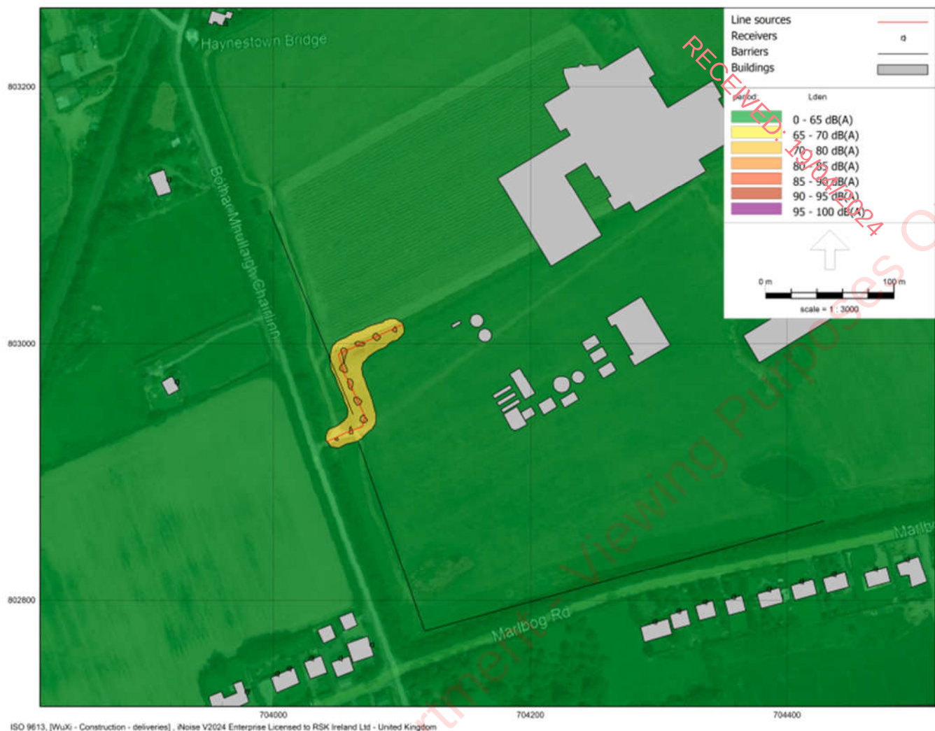
Figure 8.8 - Deliveries noise prediction contours – 65dB(A)
