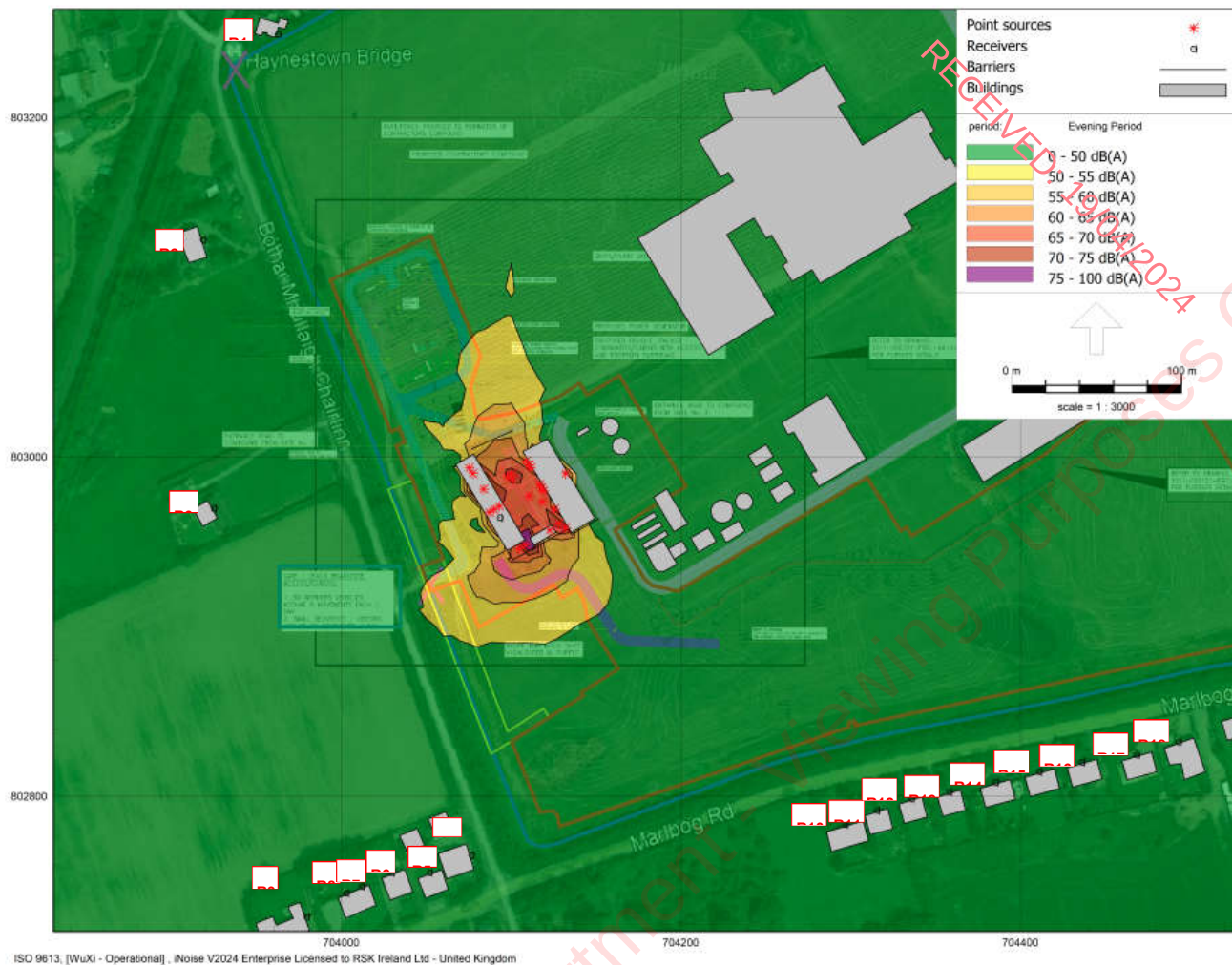
Figure 8.10 - Operational Evening-time Noise Prediction Contours – 50dB (A)
